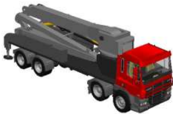
DAF Concrete Pumper
