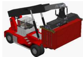
Reach Stacker with Container
